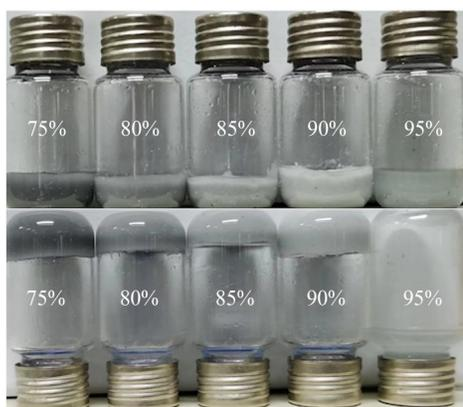
Fig. 8 Photograph of the high internal phase emulsions (HIPEs) stabilized by the CS-GNP of 0.57 wt% with different oil volume fractions.
